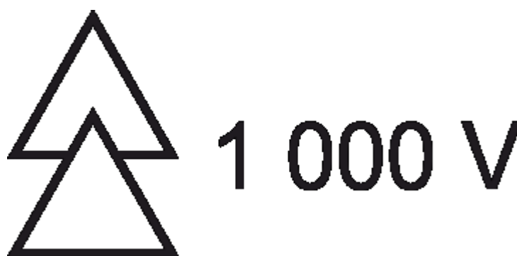
Figure 1 – Marking of the electrical working limit adjacent to the double triangle symbol (IEC 60417-5216:2002-10)
